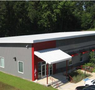
The Double-Lok® roof panel is a mechanically field-seamed, trapezoidal leg standing seam roof system. Double-Lok® panels are available in 18-inch and 24-inch widths. Double-Lok® requires a minimum slope of 1/4:12. Double-Lok® panels are ideal for industrial, commercial and architectural applications.
